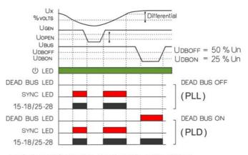
Ux = |Ugen - UBUS| (VOLTAGE, FREQUENCY + PHASE ANGLE) The differential trip levels help to prevent relay chatter as the monitored voltage level varies.
